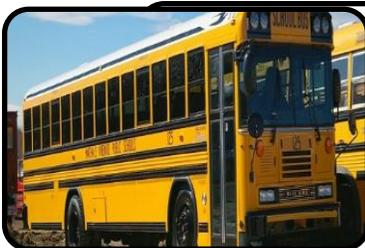
A **Type “D”** school bus is constructed utilizing a stripped chassis. The entrance door is ahead of the front wheels.
